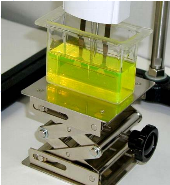
Vibration Sensor and Sample liquid
